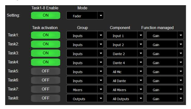
For each GPIO defined as a Fader, up to 8 tasks can be set to manage the gains on an AVDT-BOB:
