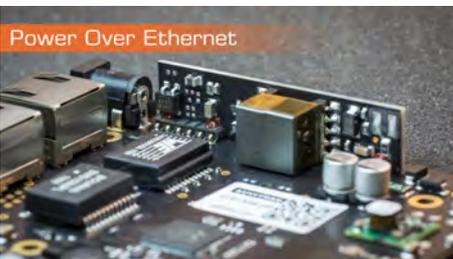
**The AVDT-BOB embeds an internal PoE module for power and communication with a single Ethernet cable.**
