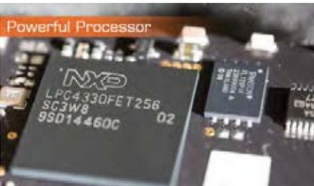
**The AVDT-BOB features a dual core ARM processor associated with a large amount of flash memory for a universal and multiplatform remote control over IP (iOS, Android, Windows, Mac OS, Linux).**
