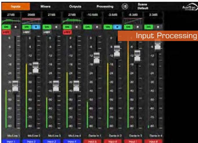
**The Input Processing block** manages up to 4 Mic/Line or digital inputs and 4 Dante inputs. It delivers 4 Direct Out (just after preamp gain or phase inverter process) and 8 processed inputs that are sent to the Mixing Processing and to the Output Processing:
