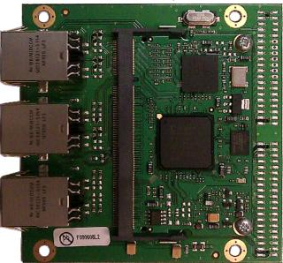
Chassis mounting is available via an optional mounting bracket and either 2 or 3 RJ-45 connector configurations. The two 2mm 40 pin connectors mounted are available either on the top (component side) or on the bottom to Maximize the flexibility in space limited applications.
